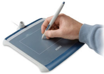
FIGURE 13.2 A pressure-sensitive drawing tablet such as this Wacom Graphire® is a must-have for serious image editing.
